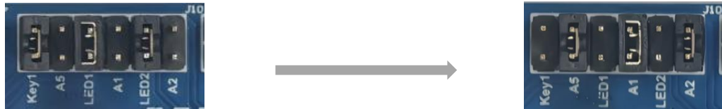
Figure 2 From Default LED1, LED2, KEY Resources to A1, A2, A5
